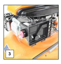
7.22 If a paper air filter is fitted, inspect and replace if necessary.
