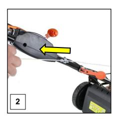
4.6 P5100SPE ONLY: Allow to run for 15 seconds, then slowly move the choke lever (1) back towards the run position.
